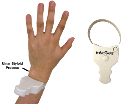
Figure 3: The AccuFitness MyoTape Body Tape Measure we used to measure the circumference of each subject’s wrist just below the subject’s ulnar styloid process.
