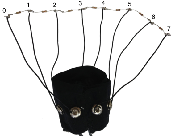
Figure 3.5.5: The resistor array used to calibrate our bioimpedance device. The 1\text{ k}\Omega \pm 5\% resistors are connected in series and act like a pseudo-wrist that can be electrically connected to the electrodes to calibrate the device. Since we measure bioimpedance at multiple electrode configurations, the reference resistance between a pair of electrodes will vary depending on the number of resistors between them. For example, the resistance between electrodes 0 4 is 4\text{ k}\Omega .
