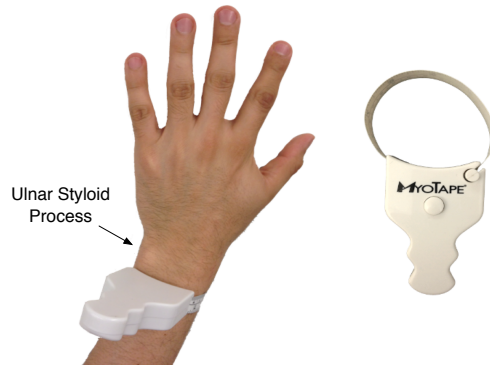
Figure 3.6.1: The AccuFitness MyoTape Body Tape Measure we used to measure the circumference of each subject's wrist just below the subject's ulnar styloid process.
