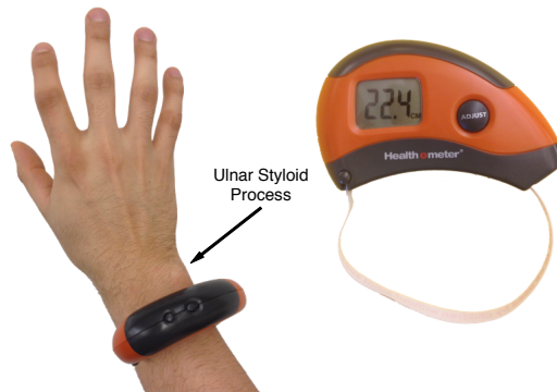
Figure 3.7.1: The Health-O-Meter Digital Tape measure we used to measure each subject's wrist circumference. It was placed just above the ulnar styloid process of the subject's non-dominant wrist where the bracelet was worn.
