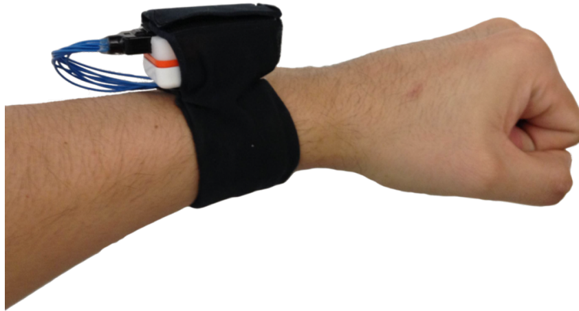
Figure 3.3.1: A subject wearing one of our bioimpedance sensors. The exposed wires connect the electrodes to our custom sensor module (which is connected to the Shimmer via the internal expansion port).
