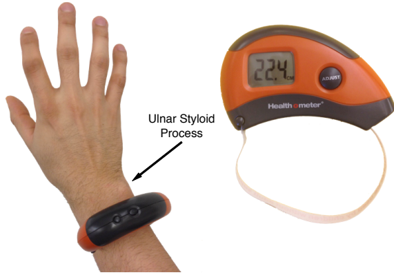
Figure 7: The Health-O-Meter Digital Tape measure we used to measure each subject’s wrist circumference. It was placed just above the ulnar styloid process of the subject’s non-dominant wrist where the device was worn.
